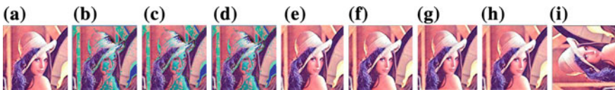
Fig. 6 Attacked images for a No attack b JPEG compression 90% c JPEG compression 80% d JPEG compression 50% e Salt and pepper 0.002 f Salt and pepper 0.003 g Wiener filter h Median filter i Rotation 90 deg
