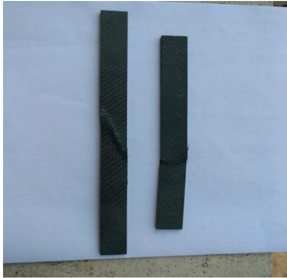
Fig. 7 Tensile failure modes
