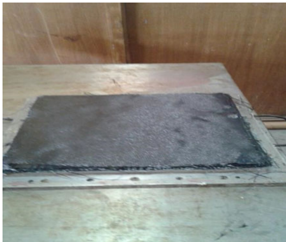
Fig. 3 Prepreg cut into 300 \times 300 mm size
