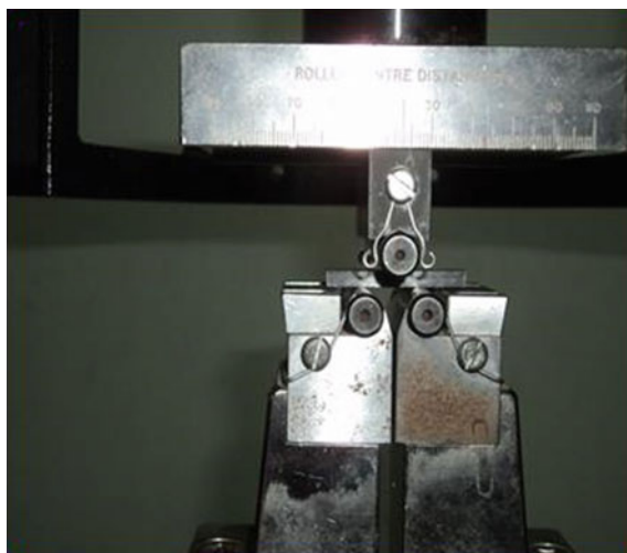
Fig. 14 Three-point bend test set-up
