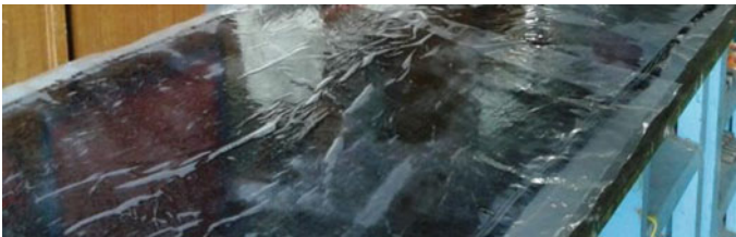
Fig. 2 Hybrid resin impregnated on carbon fabric
