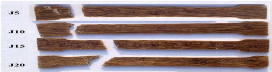
Fig. 3 Tensile specimens after testing
