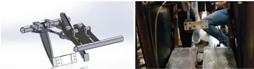
Fig. 2 Designed and practical mounting of load cell
