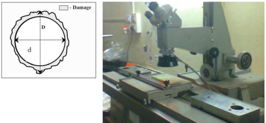
Fig. 4 Schematic diagram of delamination analysis and 2D micrometre
