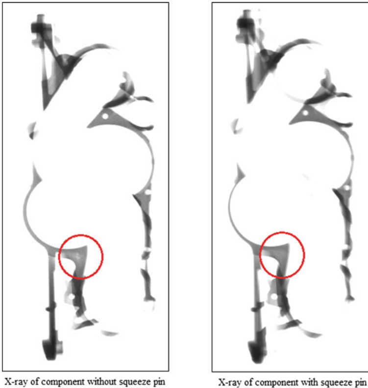
Fig. 6 Radiography X-ray inspection report with and without squeeze pin actuation
