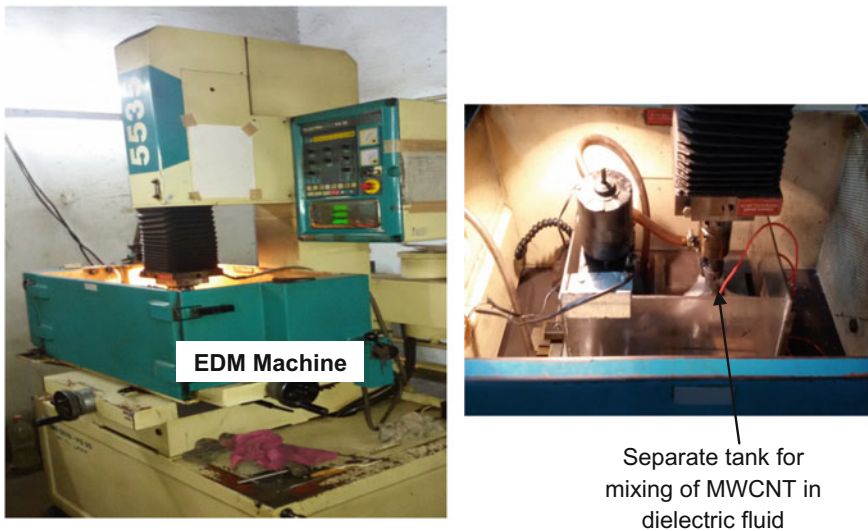
Fig. 3 Experimental setup of HA mixed electric discharge machining process
