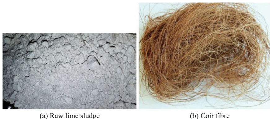
Fig. 1 Raw lime sludge and coir fibre used in the fabrication of composites
