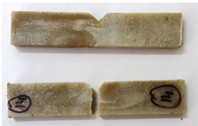
Fig. 7 A lime sludge-filled HDPE composite before and after impact testing
