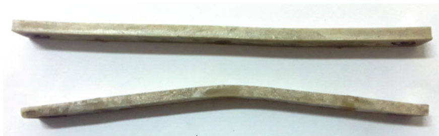
Fig. 6 A lime sludge-filled HDPE composite before and after flexural (bending) test
