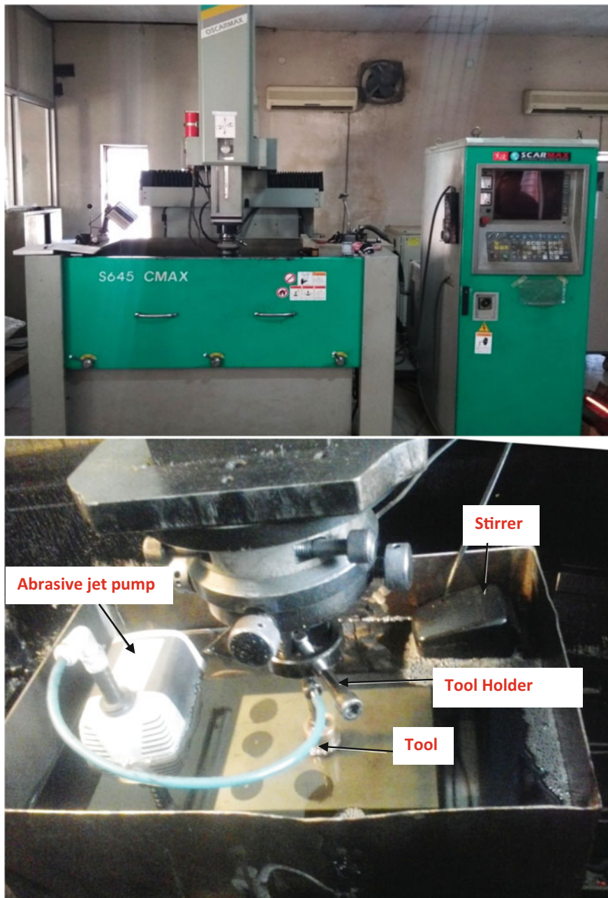
Fig. 3 EDM used for experimentation and abrasive jet machining setup
