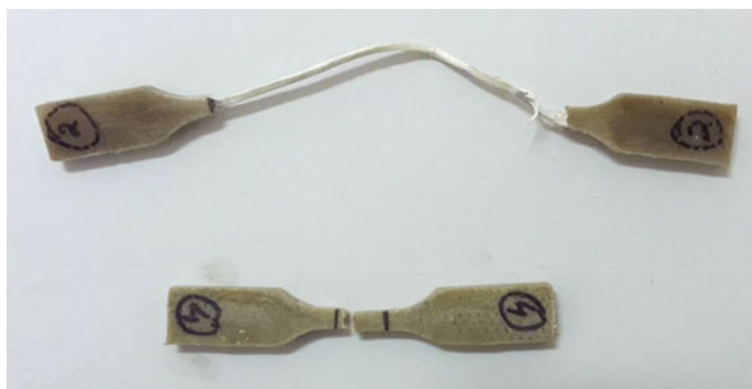
Fig. 4 A lime sludge-HDPE composite samples after tensile test having higher and lower ductility
