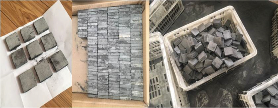
Fig. 3. Composite PCMs prepared by mix-sintering method in pilot scale: \text{Na}_2\text{CO}_3\text{-K}_2\text{CO}_3/\text{MgO}/\text{Graphite}
