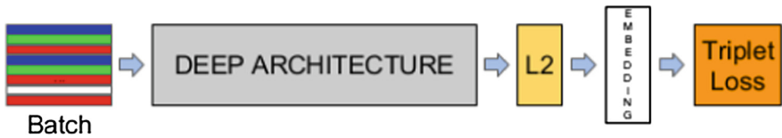
Fig. 1. Facenet Model Structure: The model contains a batch input layer and a architecture of deep CNN which is then followed by L^2 normalization that outputs the embedding of face. During training the triplet loss has been induced at the end.
