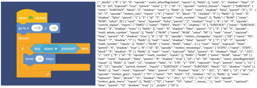
Fig. 1 A Scratch sprite (left) with several individual blocks (labeled “go to”, “forever”, etc.) and its corresponding textual representation in JSON (right)
