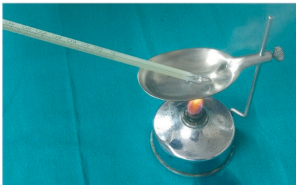
Fig. 3 Preparation of anhydrous glycerol using a burner along with a thermometer to measure the temperature continuously
