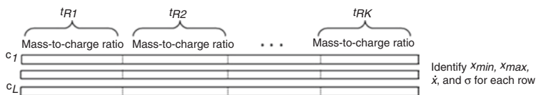
Fig. 19.4 Identify the minimum, maximum, mean and standard deviation of each row
