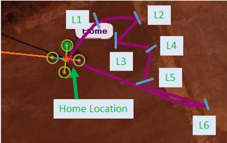
Fig. 8 UAV returns to home location while exceeding the threshold range at L 6
