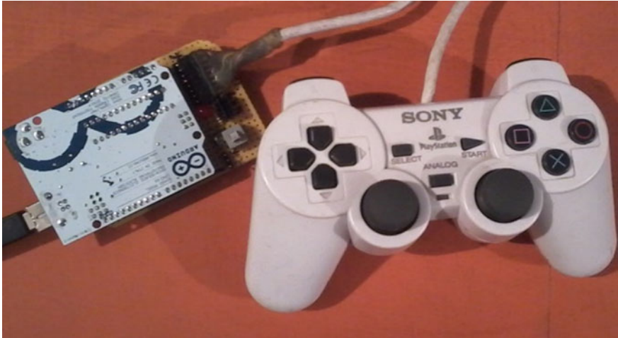
Fig. 8 PS-2 interfaced with Arduino
