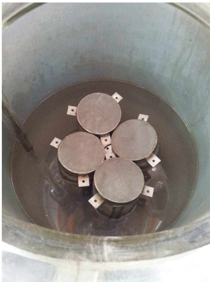
Fig. 3 The mesh containers containing palm wastes are immersed in bioethanol
