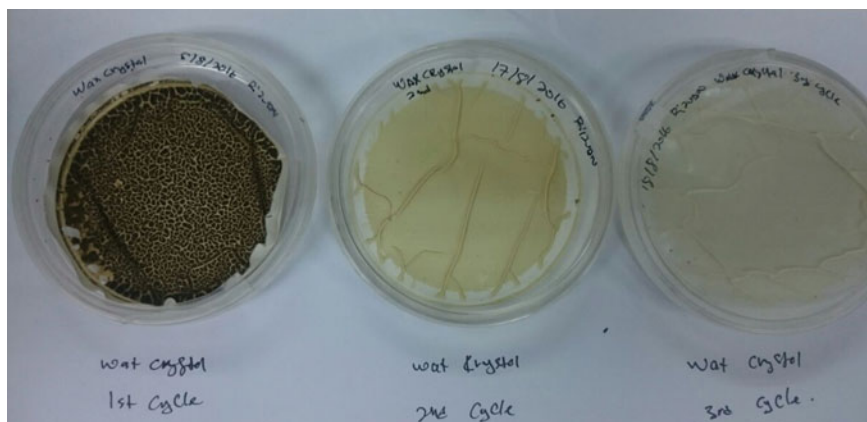
Fig. 10 The three-step fractionation crystallisation experiment using the liquid residue of the filter of the single-batch crystallisation experiment furthered yielded a better looking palm wax with its distinctive gold colour. In the second cycle sample, there was a better palm wax and consequently in the third cycle ultrafine nanosized palm wax was recovered
