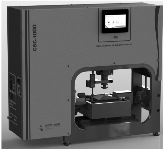
Fig. 3. View of the compact conventional direct shear equipment.
