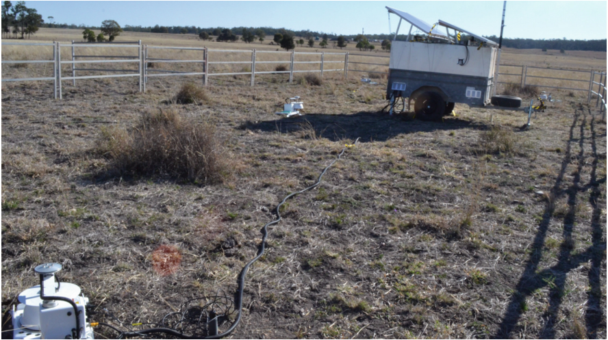
Fig. 1. A solar powered monitoring station for atmospheric and soil-gas flux chamber measurements deployed onto a mobile trailer.
