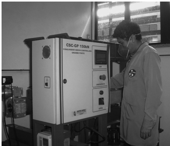
Fig. 4. View of direct shear equipment of large size automated.
