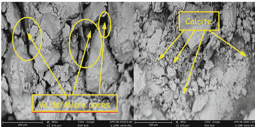
a) Natural lateritic soil (b) Treated Lateritic soil ( 1.2 \times 10^9 / ml S.pasteurii suspension density)
