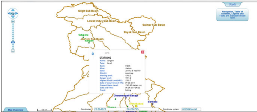
Fig. 23.6 CWC portal showing river gauge data for Sangam, Jammu, and Kashmir station
