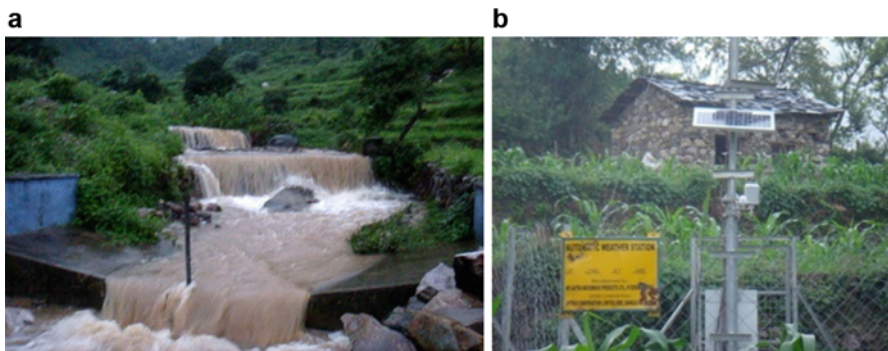
Fig. 17.1 (a) Surface runoff gauging structure, (b) Automated Weather Station (AWS), Dehradun, India
