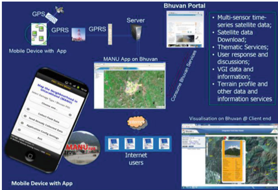
Fig. 25.2 System architecture of MANU. (Source: Murthy et al. 2014)
