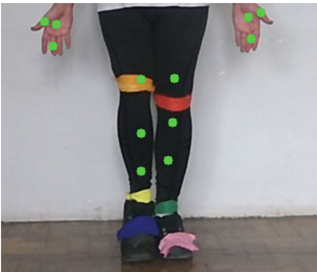
Fig. 1 Six color markers and black legging pants. Green dots indicate joints captured by Kinect standard method (Color figure online)
