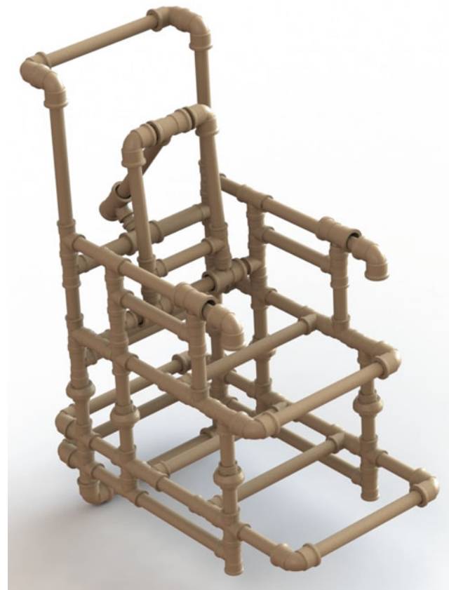
Fig. 1 3D rendering of child's electric wheelchair frame made by PVC pipes and Arduino
