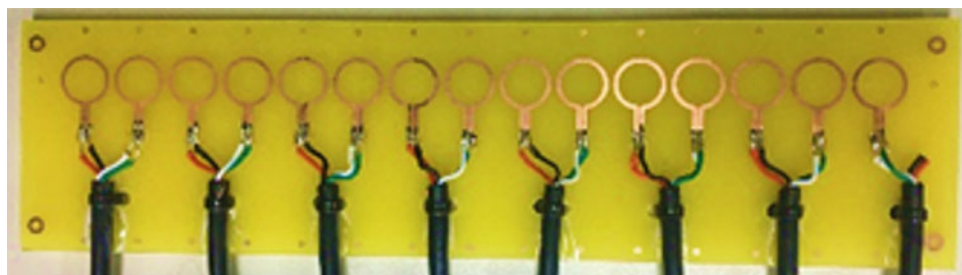
Fig. 1 Multi-channel measuring system with 15 sensor coils, 5 mm median radius, and 1.2 cm distance between centers of sensor coils
