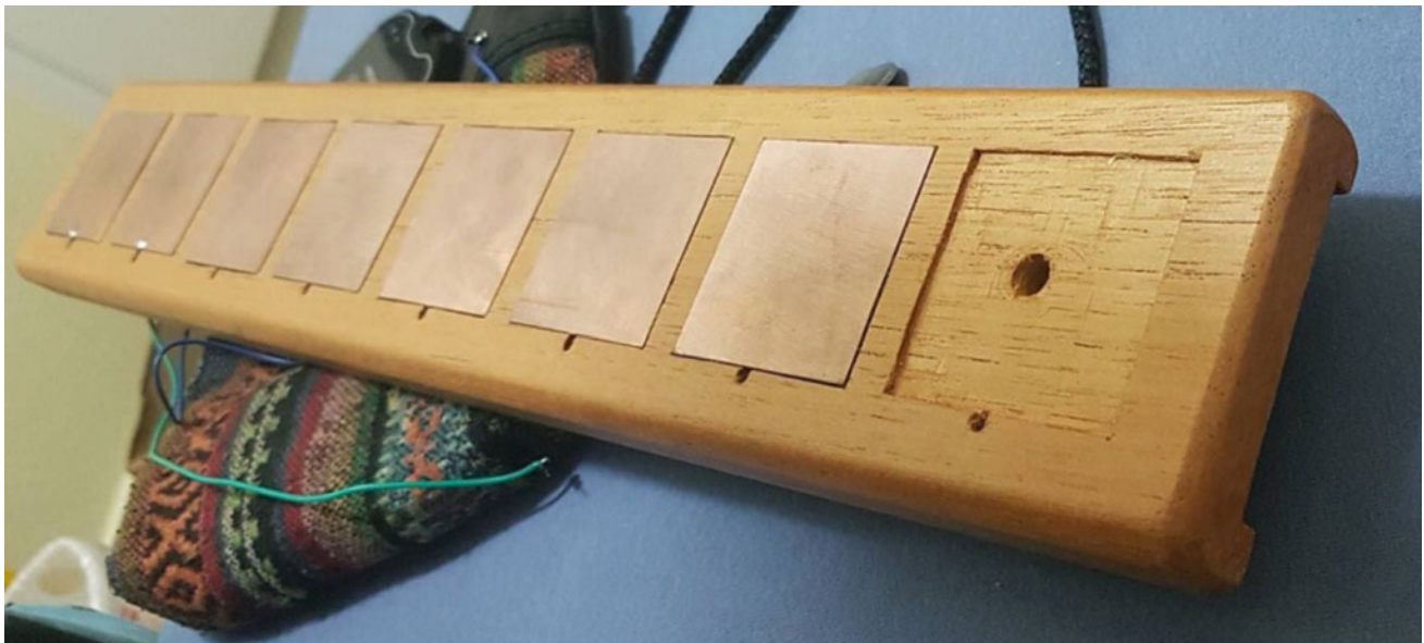
Fig. 2 Partial assembly of the sensors into the wooden board. Notice the big hole in the middle of the sensor groove for passing the ground wire and the small hole next to the groove's edge for passing the active sensor wire
