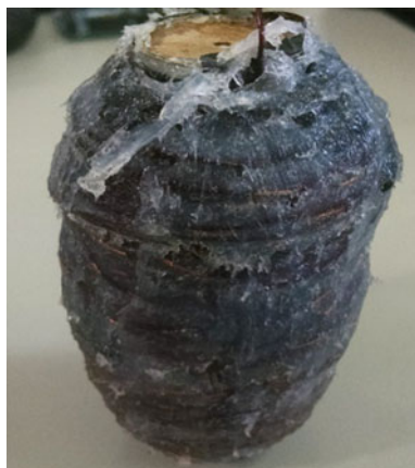
Fig. 9 Electromagnet prototype covered with silicone
