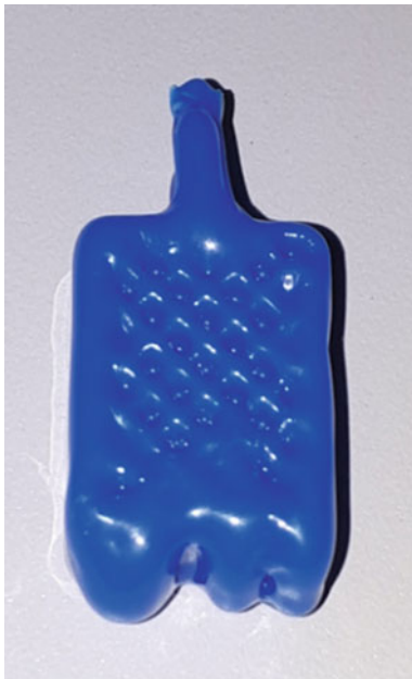
Fig. 6 Excessively melted surface of horizontally printed part, 60 min treatment
