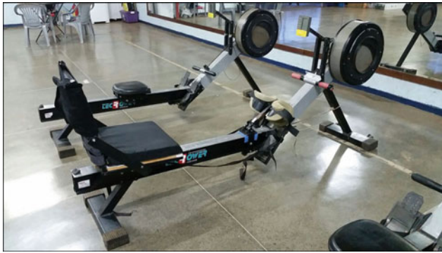
Fig. 3 Comparison between the adapted rowing machine and an untouched original one. Note the seat for trunk stabilization, the custom device for legs stabilization, and the safety straps
