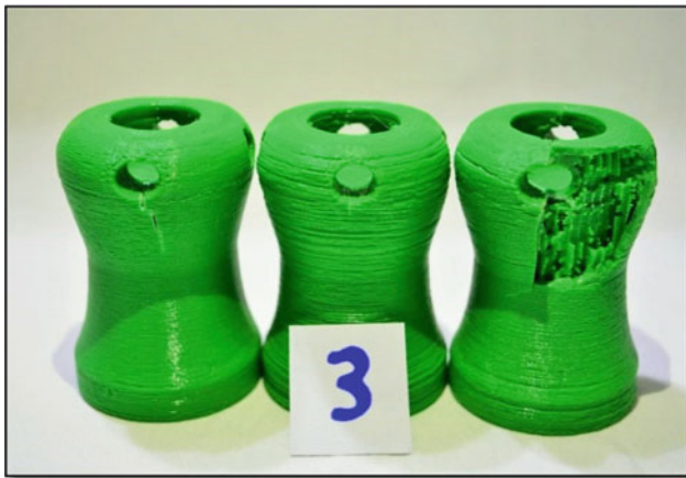
Fig. 9 Adapter models for lower limb prosthesis after compression test
