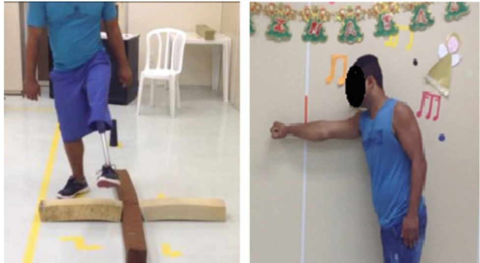
Fig. 2 The obstacle test (left) and the slop test (right), both using the mechanical prosthesis
