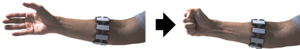
Fig. 1 Myo Armband device worn on a user's forearm executing relaxed to Full Fist position exercise
