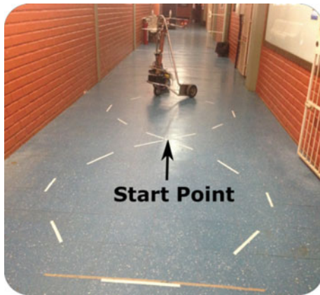
Fig. 3 Experiment where the subjects were asked to follow a lemniscate curve indicated on the floor
