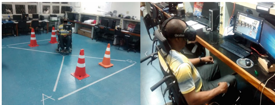
Fig. 1 Participant testing the real EPW (left) and the virtual one in the SimCadRoM (right)
