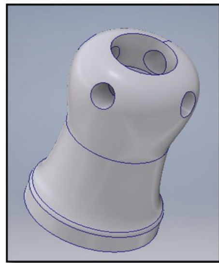
Fig. 2 Adapter model for lower limb prosthesis created in inventor software
