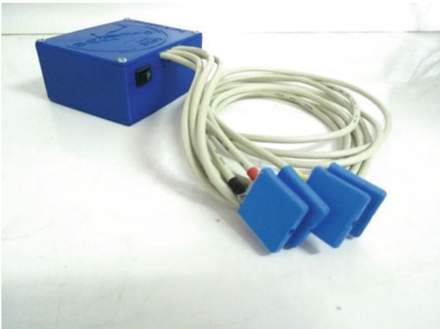
Fig. 2 Motion detection, processing and sending via Bluetooth
