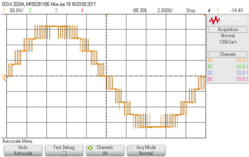
(b) Hardware result of voltage and current (1-cycle) of proposed 9-level Inverter.
