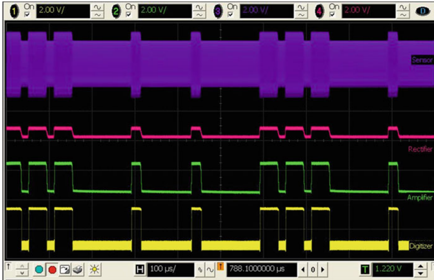
Fig. 7.25 Waveforms of the outputs of four main blocks: blue, purple, green, and yellow waveforms are the output of the sensor, the rectifier, the amplifier, and the digitizer, respectively
