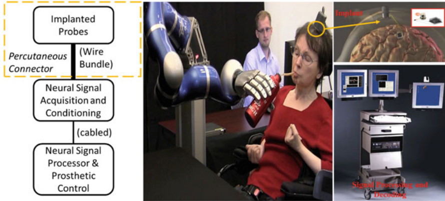
Fig. 9.1 A block diagram view of a multi-channel neural recording system for brain-computer interface applications. Multi-channel implantable microelectrode arrays are connectorized using wire bundles, and external cabled electronics and computers are used for signal acquisition and processing
