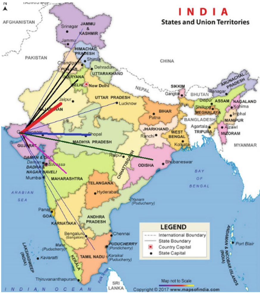
Fig. 1 Desire line diagram of truck trips from Kandla port
