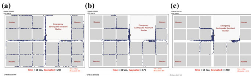
Fig. 9 Sequential simulation snapshots for 2000 agents consisting 100% males
