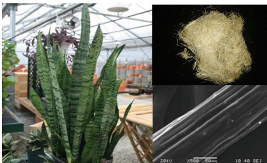
Fig. 4 Sansevieria roxburghiana plant, fibre and SEM image
