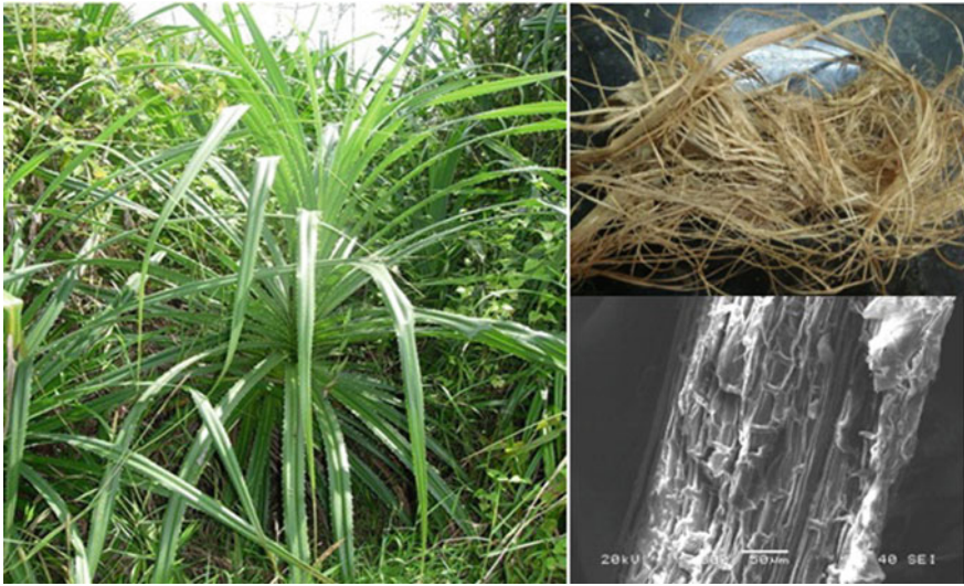
Fig. 5 Pandanus odorifer plant, fibre and SEM image
