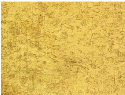
(e) Microstructure SS 304 base metal with 200× magnification
