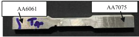
Fig. 7 Top view of welded specimen
