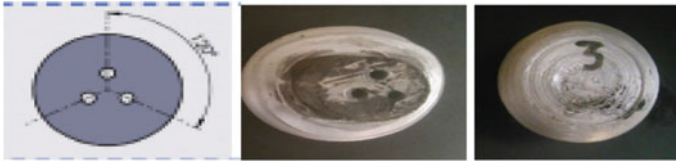
Fig. 3 Conceptual pattern of adding MMC particles in consumable rod
