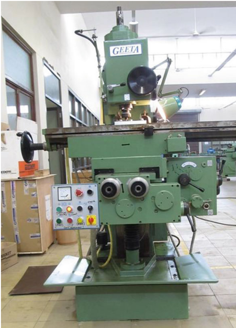
Fig. 1 Setup for FSW on special purpose VMC (available at PDPU Welding Research lab under the sponsored project of ISRO E33011/60/2010-V)
