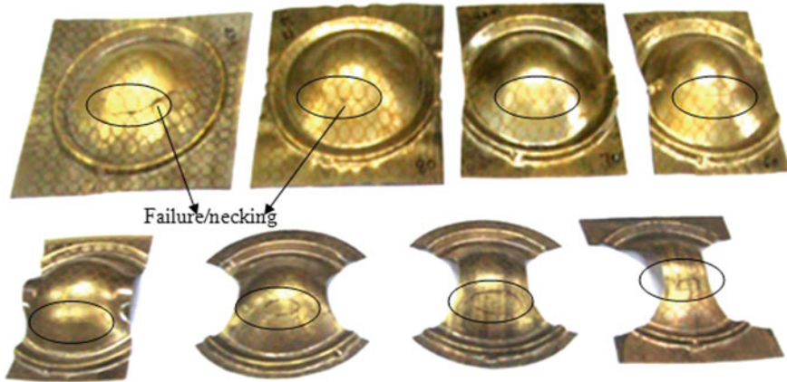
Fig. 5 Specimens of different width tested for the determination of FLD
