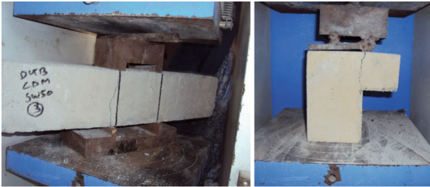
Fig. 9 Crack pattern of the specimens for JSFC-SF6 and Bairagi and Modhera method
