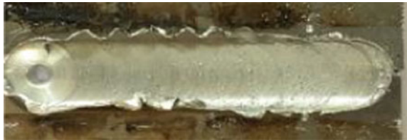
Fig. 2 Top view of welded specimen
