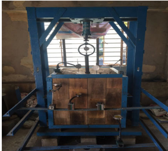
Fig. 3 Reinforced earth wall test model
