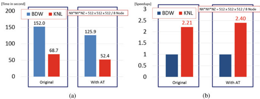
Fig. 2.18 Effect of AT and comparison of execution time. It shows aggregated execution time of kernel update_stress up to 2000 time steps. (a) The best execution time between BDW and KNL between original and with AT. (b) Normalized speedup factors of the KNL based on execution time in the BDW
