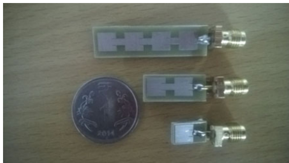
Fig. 12 Fabricated antenna using Fr-4 substrate
