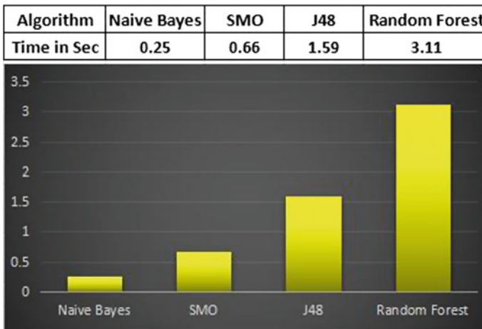
Fig. 9 Graphical representation of all classifiers on the basis of time requirements (X-axis represents used classifiers and Y-axis represents time taken to build classifiers)
