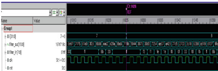
Fig. 7 Simulation results for 4-tap pipelined DA-based adaptive FIR filter
