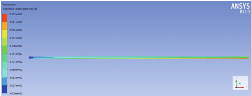
Fig. 4 Temperature distribution along wall
