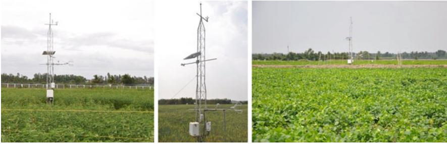
Fig. 2.3 Eddy covariance-based GHG measurement in dhaincha ( Sesbania spp.), wheat and soybean ecosystems in the years 2013 and 2014
