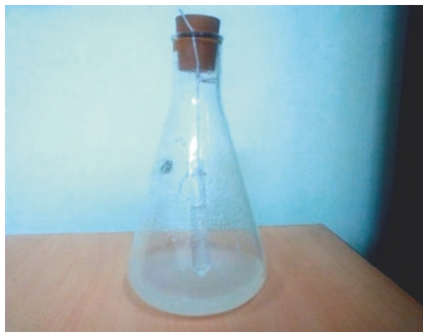
Fig. 24.5 Reaction setup of CO 2 evolution assay showing the hanging tube containing 0.1(N) NaOH
