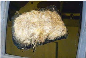
Straw is inoculated with fungal mycelium which is absorbing oil from water
