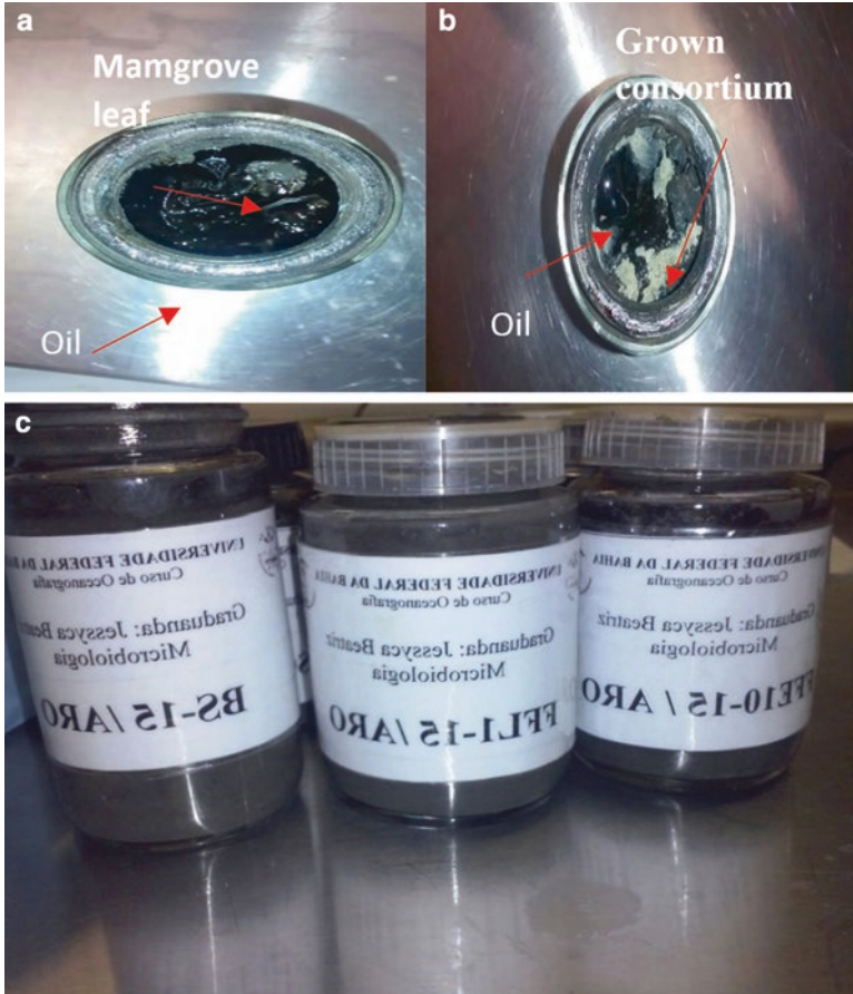
Fig. 11.21 Assembling the experiment: (a) glass pots with sediment and mangrove leaf; (b) capsules with immobilized consortia; (c) assembled experiment. (Source: Palmeira 2014)
