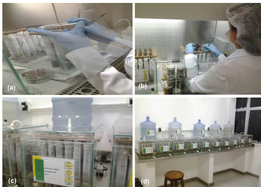
Fig. 11.6 Stages of the experiment. (a) Inoculation of the capsules, (b) simulation of the oil spill, (c) capped and sealed simulation unit, and (d) mounted bioaccumulation system. (Source: Lima 2014)
