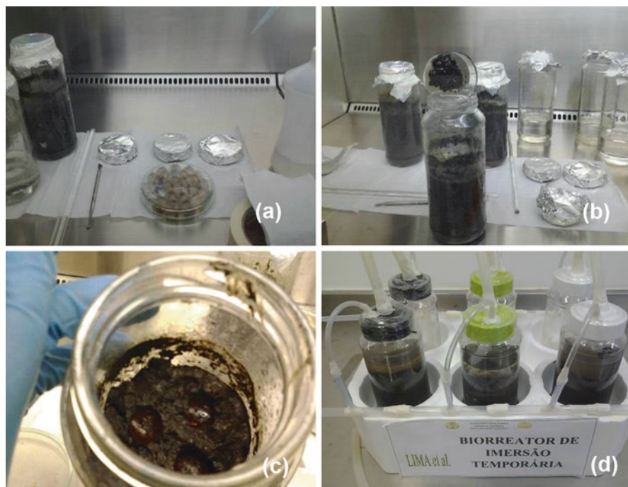
Fig. 11.13 Assembling the experiment: (a) capsules with immobilized consortia, (b) simulating oil spill, (c) top view of the bioreactor, and (d) assembled prototype. (Source: Lima, 2014)
