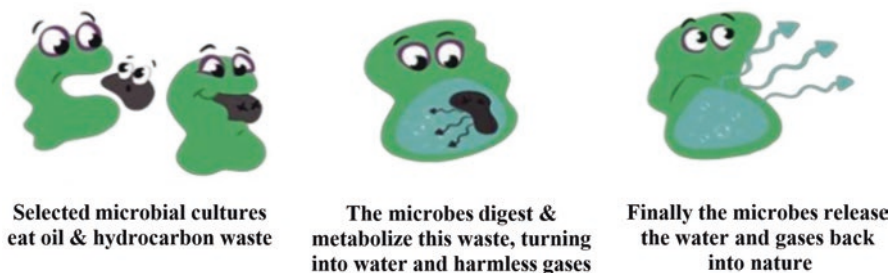
Fig. 17.1 Illustration of biodegradation of oil in soil by selected microbial cultures in the environment. (Sources: NCEPI)
