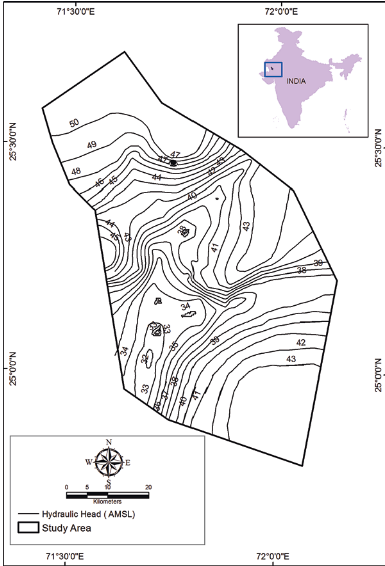
Fig. 12 Variation of hydraulic head of unconfined aquifer
