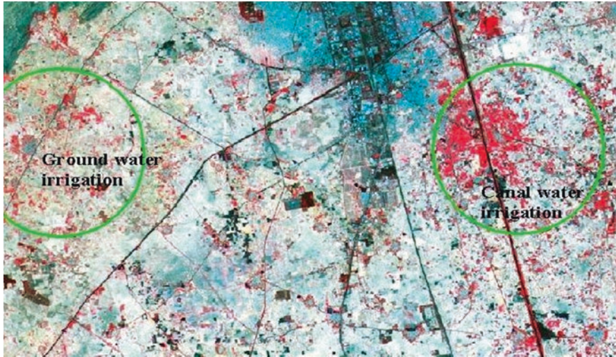
Fig. 2 IRS LISS II false color composite image indicating areas irrigated through groundwater and canal water in Faridabad district, Haryana
