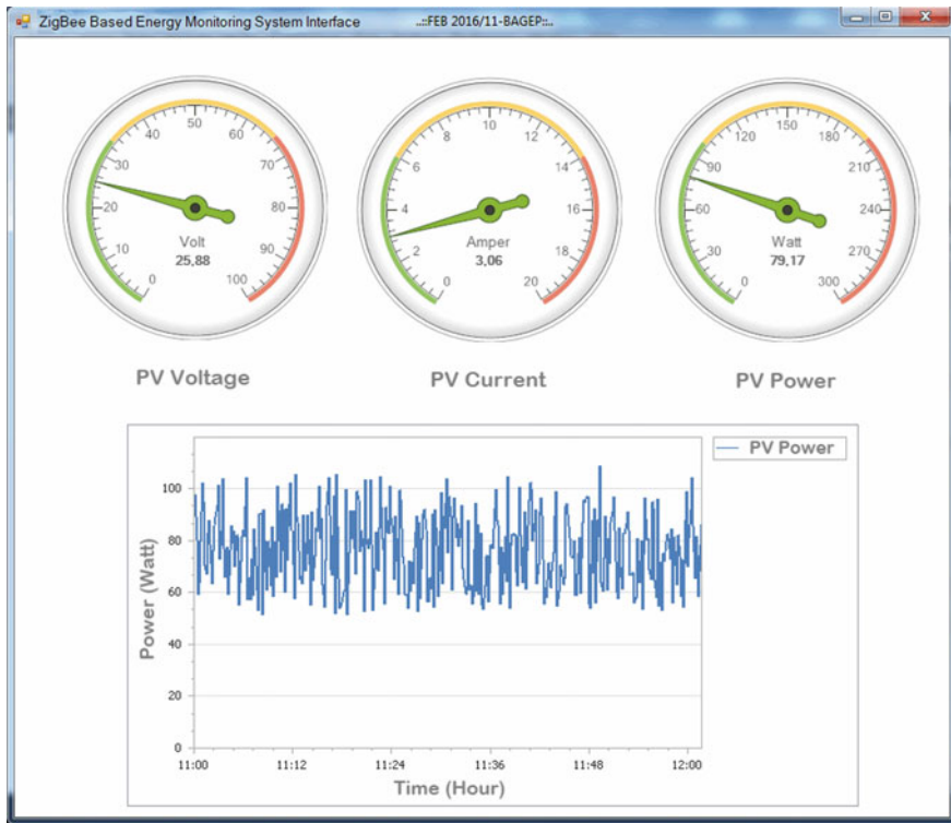
Fig. 15.8 A screenshot of ZigBee-based remote energy monitoring system [30]
