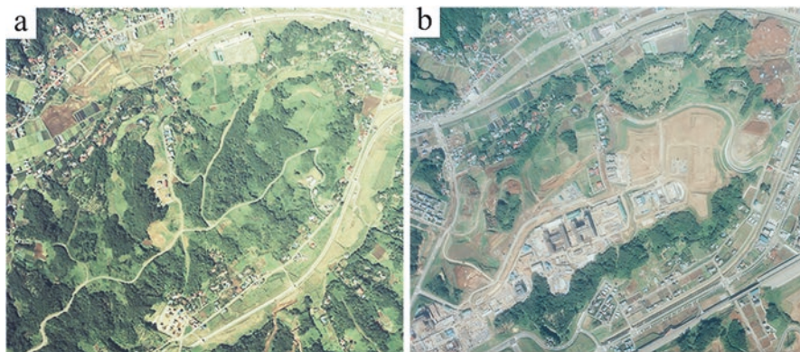
Fig. 1.13 Aerial photos of land use change at Minamiosawa from (a) 1979 to (b) 1989. The hill top has been removed to flatten the area for construction of buildings. Cut and banking also took place for land leveling. Soils have been disturbed through the process of construction. Photos from Geospatial Information Authority of Japan. (GSI: a; CKT841-C28-18, b; CKT841-C28-18)
