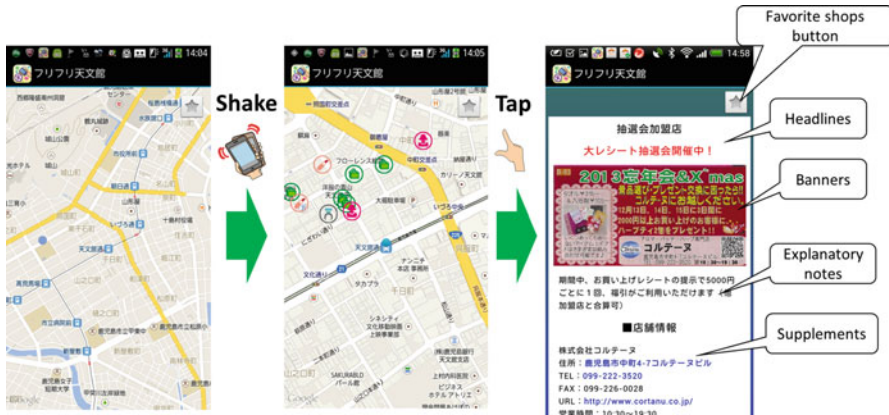
Fig. 20.5 Shake and tap for searching and focusing and the forms of information contents
