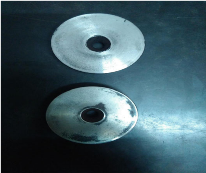
Fig. 5 Boronized En19 disc after wear test
