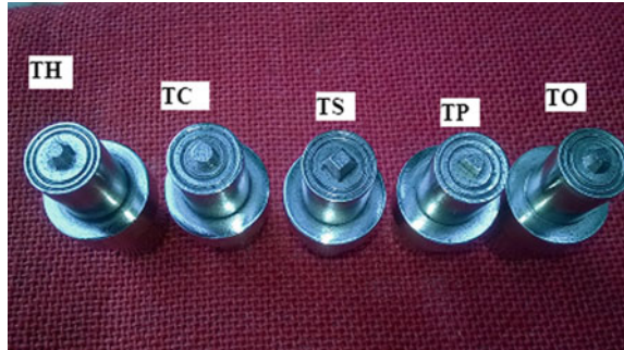
Fig. 1 Photographic view of FSW tools
