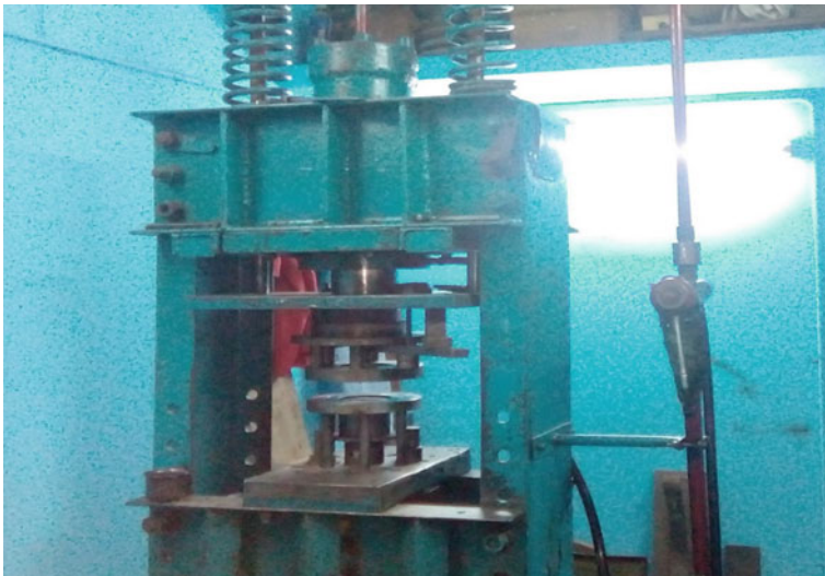
Fig. 4 Deep drawing machine
