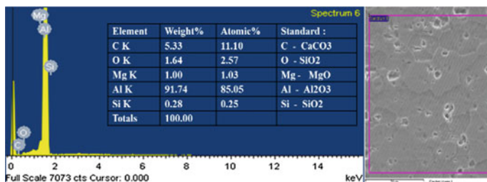
Fig. 9 EDS analysis of Al/Al 2 O 3 surface nanocomposite
