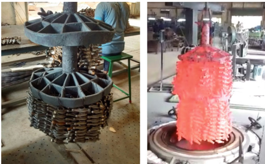
(a) Circular fixture with suspended grey cast iron rocker arm
