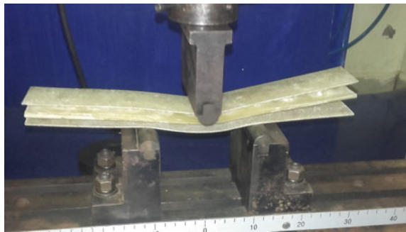
Fig. 3 Three-point bend test setup for loading the specimen
