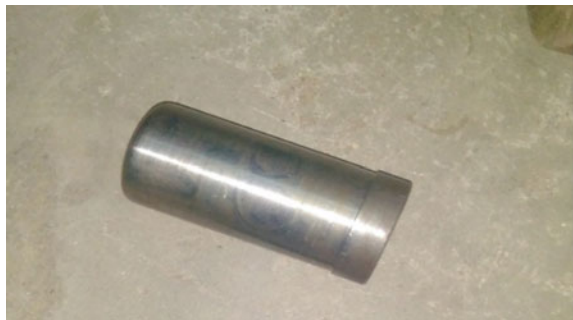
Fig. 3 Deep drawing punch
