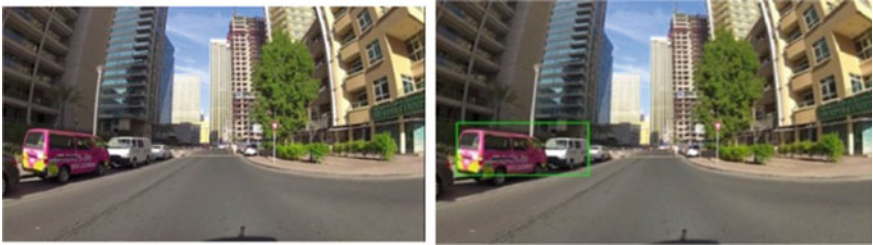
Fig. 6 Detected vehicles with Gabor+CNN system
