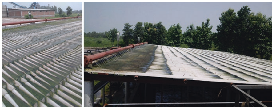
Fig. 19.4 Slope – illumination – aeration panel of algal ETP – large scale at Pasupati Acrylon
