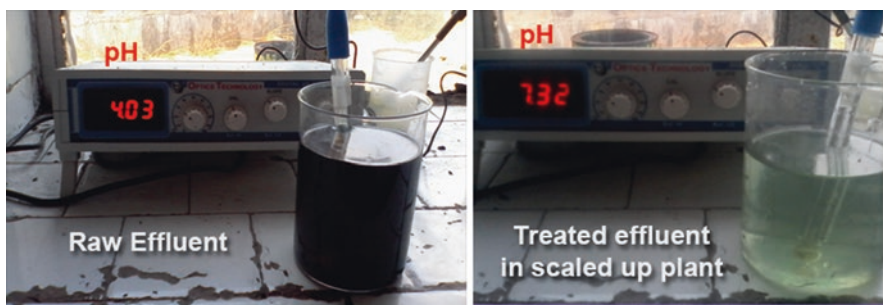
Fig. 19.6 Comparison of treated effluent with raw effluent – Pasupati Acrylon
