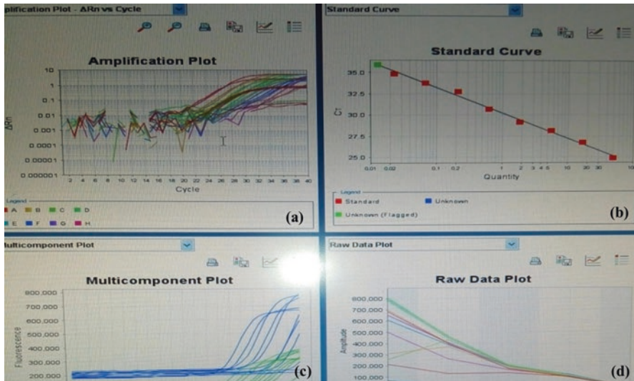
Fig. 3.5 Parameters calculated during the process of quantitative real-time PCR, i.e., (a) amplification plot, (b) standard curve, (c) multicomponent plot, and (d) raw data plot
