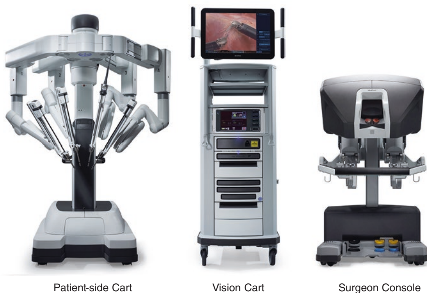
Fig. 11.1 da Vinci Si system. Images are duplicated with an authorization for publications to make duplicate copies for editorial use only. © [year] Intuitive Surgical, Inc.
