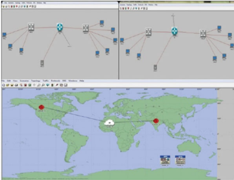
Fig. 4 Local and long distance VoIP call model in LAN
