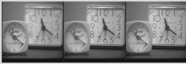
Fig. 1 Multi-focus image: source-picture 1, source-picture 2, and CSR output
