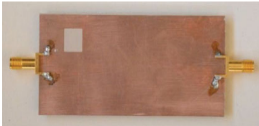
Fig. 5 Bottom view of fabricated layout of proposed model with 1st iteration DGS
