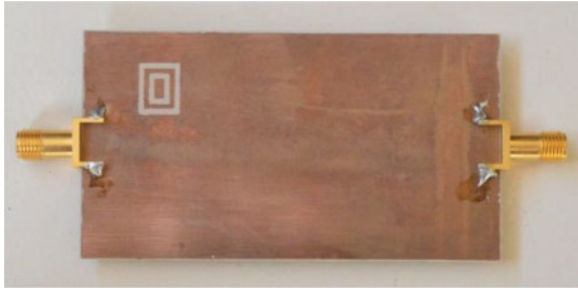
Fig. 6 Bottom view of fabricated layout of proposed model with 2nd iteration fractal DGS
