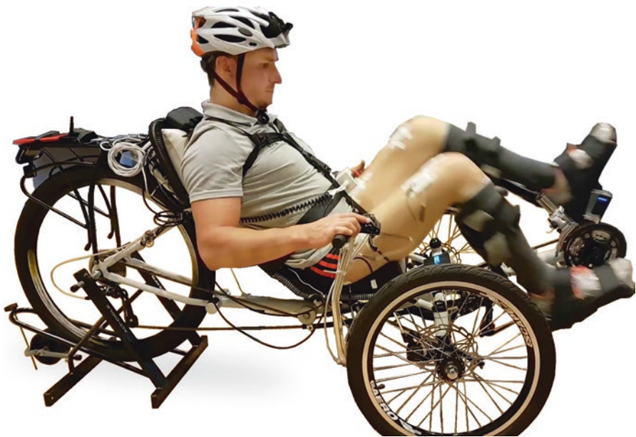
Fig. 26.5 FES-assisted cycling system developed by our group to compete in the Cybathlon 2016 whose development detail was published in the IEEE Robotics and Automation Magazine [94]
