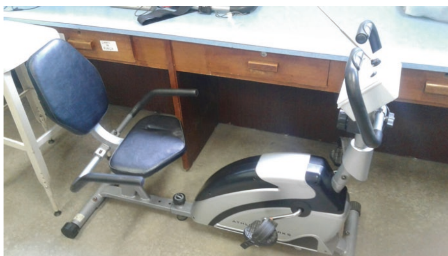
Fig. 26.8 Stationary cycle ergometer system in process of developing by our research team to explore protocols of FES-assisted cycling for poststroke hemiparesis people
