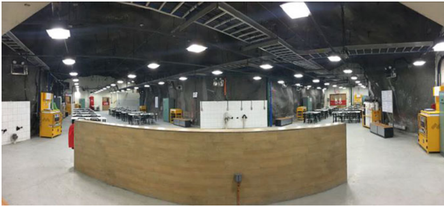
Fig. 6. Dual-purpose 250-person lunchroom/refuge chamber at the GBC mine
