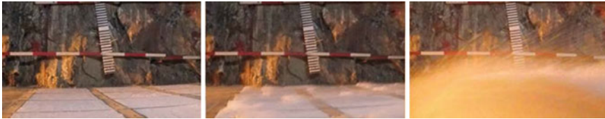
Fig. 9. Scouring of wet-applied, then dried rock dust. The images center and right clearly show chunks of agglomerated dust
