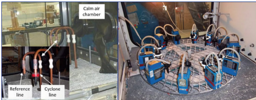
Fig. 4. Cyclone sampler efficiency testing (left) and dust concentration test set up [40]
