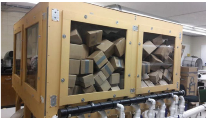
Fig. 7. Empty boxes of different sizes used to simulate broken rock mass
