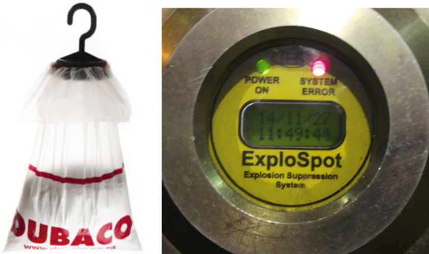
Fig. 6. Error indication and commissioning of passive and active barriers
