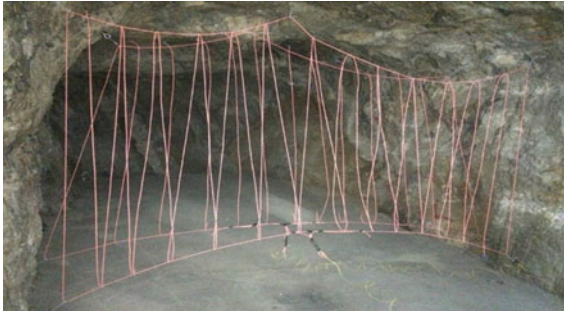
Fig. 3. Detonation cord lattice for a medium-sized blast
