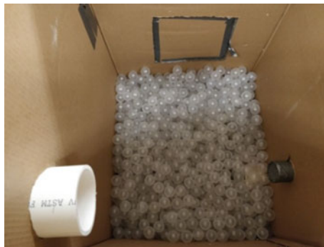
Fig. 10. Model filled with one layer of balls (1.5-inch dia.)
