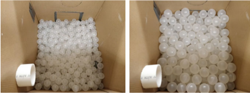
Fig. 11. Model filled with three layers of balls (1.5, 2, 2.75 inches in diameter)
