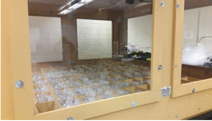
Fig. 5. Plastic balls of different dimensions were used to fill the model
