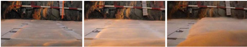
Fig. 8. Scouring of dry-applied, dry rock dust
