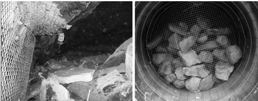
Fig. 1. Left—Image of Western U.S. Longwall void [13]. Right—Image of simulated gob used by CSM researchers
