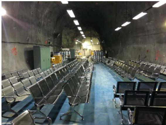
Fig. 12. 300 person refuge chamber in the DMLZ mine
