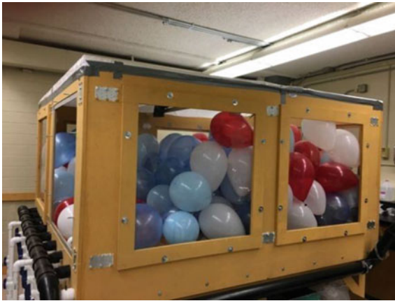
Fig. 6. Balloons of varying sizes were used to simulate the broken rock mass
