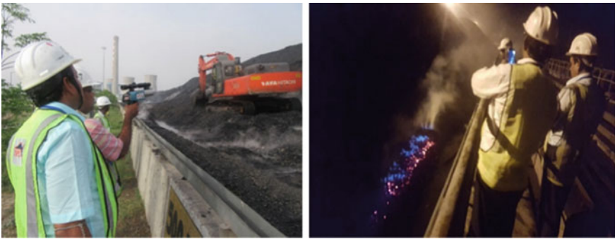
Fig. 3. Thermal survey using infrared gun at yard no 202
