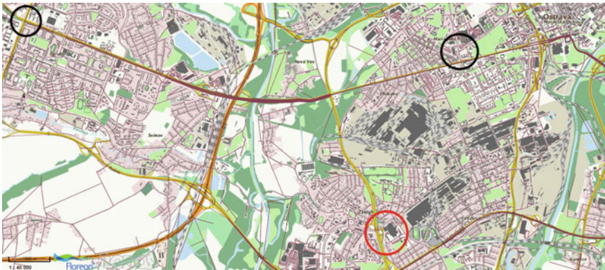
Fig. 5 Visualized betweenness centrality output for a part of Ostrava city. In black circles, there are selected vertices with value \beta = 1 , and in red circle there is a selected vertex with value \alpha = 1 (color figure online)
