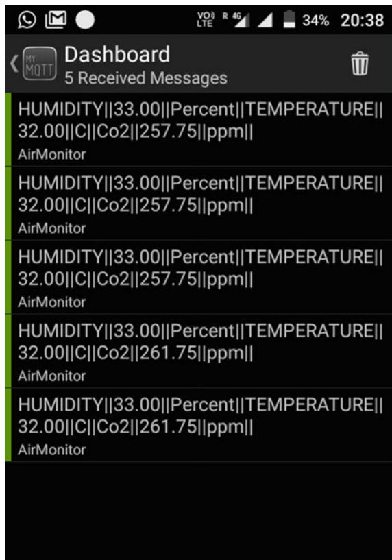
Fig. 9 Client has made subscription to topic “AirMonitor” over MQTT broker, after successful subscription acknowledgement by the broker, it starts receiving message over MQTT lens (Web Client Utility)
