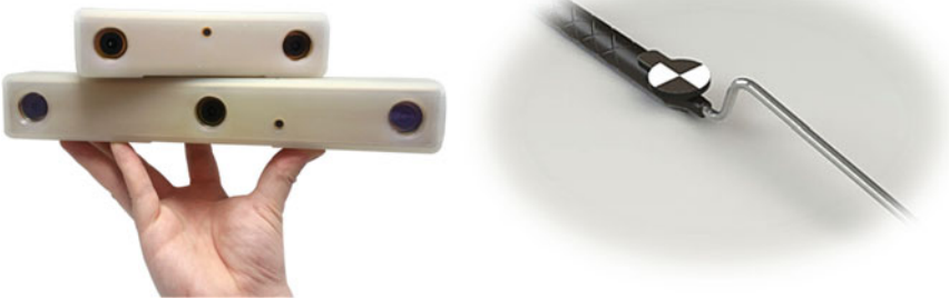
Fig. 4.4 Available MicronTracker models and the ClaroNav tool (an ergonomic probe handle with two permanent targets). (Image courtesy of ClaroNav, Toronto, Canada)
