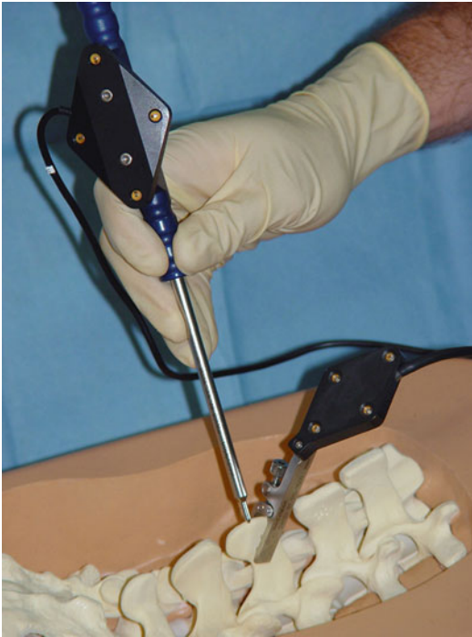
Fig. 1.6 Dynamic reference base. A dynamic reference base allows a navigation system to track the anatomical structure that the surgeon is operating on. In the case of spinal surgery, this DRB is usually attached to the processus spinosus with the help of a clamping mechanism. It is essential that it remains rigidly affixed during the entire usage of the navigation system on that vertebra
