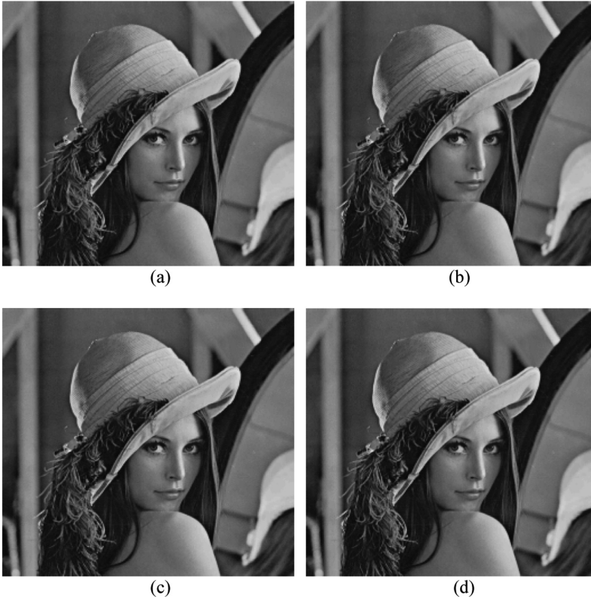
Fig. 8. The reconstructed images using all examined techniques (a) FIC-QP-CC (28.90 dB) (b) FIC-QP-DWT (28.86 dB) (c) FIC-AQP-AC (29.36 dB) (d) FIC-AQP-CC/FIC-AQP-HC/FIC-AQP-MHC (29.31 dB)
