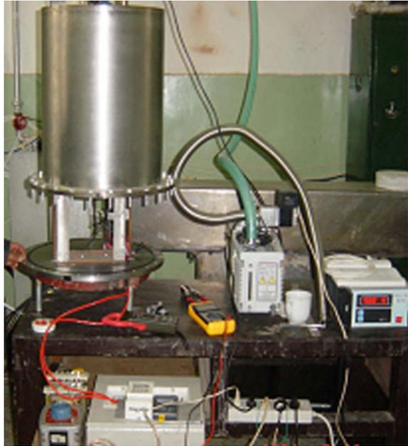
30 A. However, the steady equilibrium temperature is 305 °C when the environment pressure is 100 Pa and current is still 30 A.
