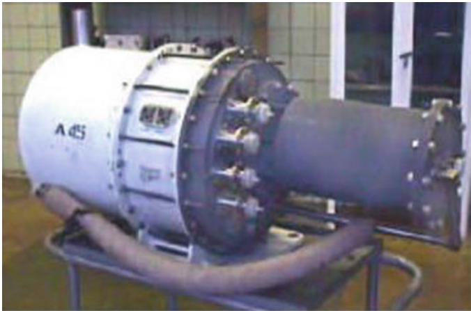
Fig. 1 The photo of POLIZON furnace, reprinted from reference [2]. Copyright 2018, with permission from Acta Astronautica
