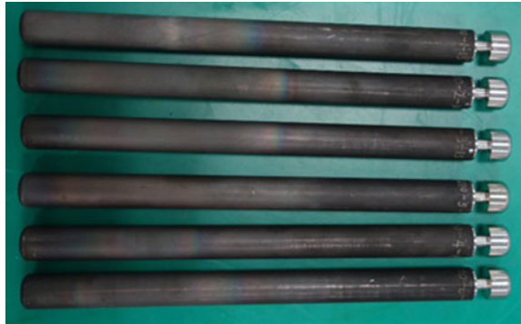
Fig. 6 The returned sample cartridges in MMP facility served on the Chinese SJ-10 recoverable satellite
