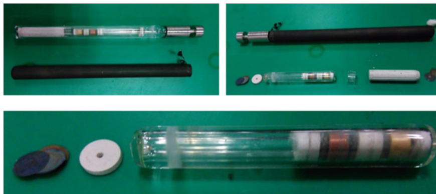
Fig. 13 Recovery and dismantling diagram of ampoule sample
