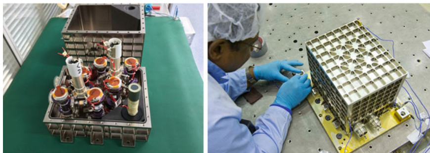
Fig. 2 Left: The six HP cells contained in the C-box. Right: The C-box once closed
