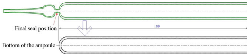
Fig. 3 Schematic diagram for packaging of vacuum type quartz ampoule
