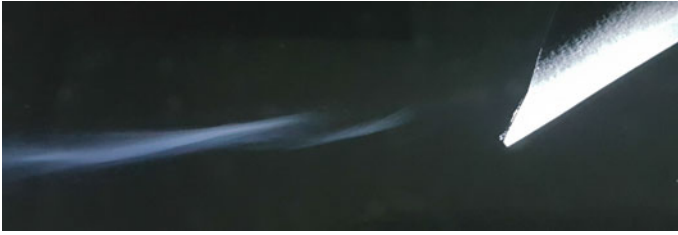
Fig. 4 Visualization: the vortex generated from inside the wing is spread outside
