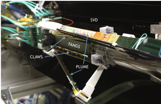
**Fig. 2.** The vertex detector dedicated for SuperKEKB commissioning Phase 2. The integration was tested at DESY, the thermal interference was quantified and the integration sequence was decided. During the test, SVD, FANGS, CLAWS and PLUME were involved.
