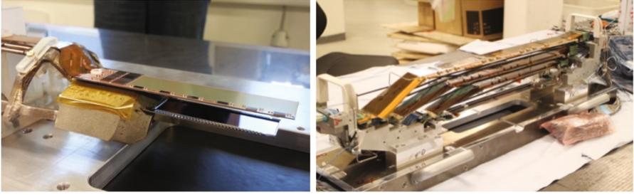
**Fig. 1.** The 2-layer PXD modules and 4-layer SVD modules tested in the test beam at DESY.
