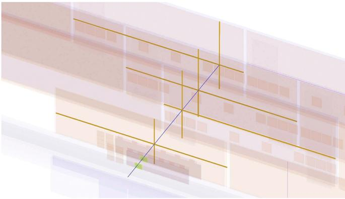
**Fig. 3.** An event display in the test beam at DESY. The blue curve is the reconstructed track, the yellow lines indicated the fired SVD strips, and the green regions are the determined ROI on the PXD.
