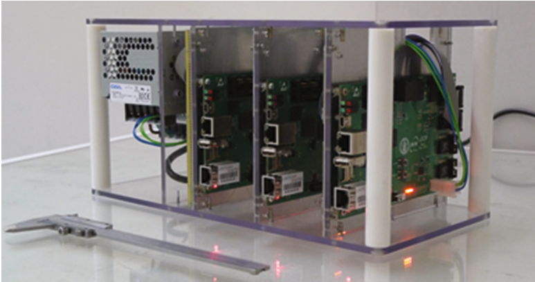
Fig. 1. The uSOP board in a 3-slot minicrate
