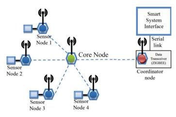
Fig. 2 Functional diagram of IWSN
