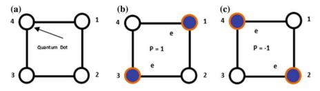
Fig. 1 a A typical 4-dot QCA cell, b logic '1' encoding, and c logic '0' encoding
