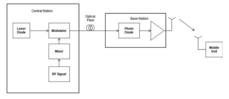
Fig. 2 RFoF downlink system architecture
