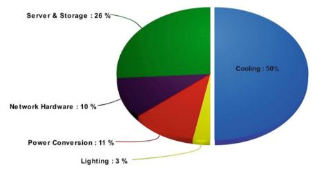
Fig. 1 Power consumption breakdown of a datacenter [16]
