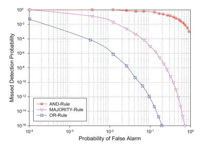
Fig. 2 CROC curves of hard fusion rule in AWGN channel
