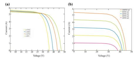
Fig. 1 I-V characteristics of PV panel a at variable irradiance b at variable temperature
