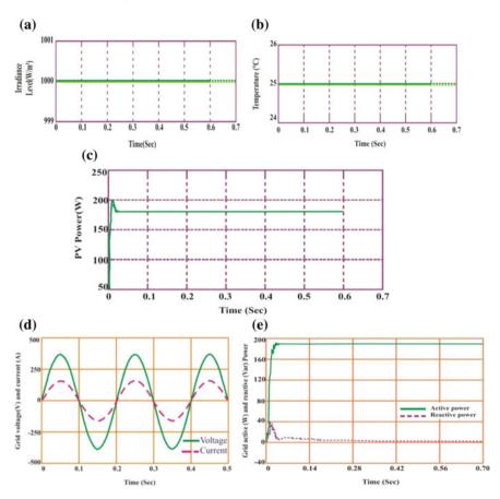
Fig. 5 Simulated responses of **a** irradiance level **b** temperature **c** PV power **d** grid voltage **e** active and reactive power
