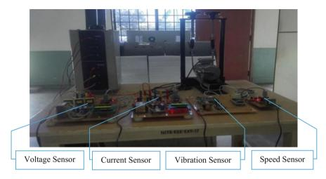
Fig. 4 Experimental setup (on sensor node)
