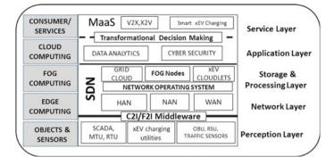
Fig. 2 Service-Oriented Architecture (SOA) of FOG computing model in a Smart Grid-based transportation system
