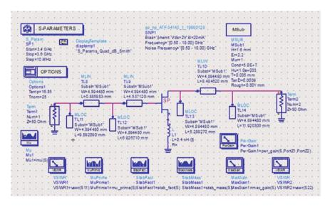
Fig. 15 LNA design with source inductor
