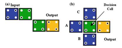
Fig. 3 a An inverter configuration, and b 3-input majority gate
