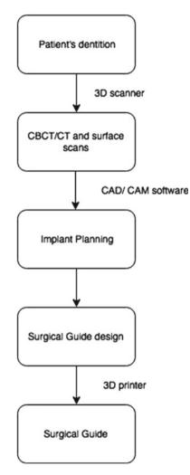
Fig. 1 General methodology for fabricating surgical guides
