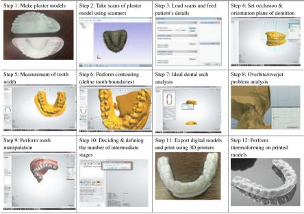
**Step 2: Take scans of Plaster Model using Scanner**: These models are scanned using 3D scanners to obtain digital data (.stl) which is given as an input to software for processing. An alternate to decrease the overhead of making plaster models is the recent technique of scanning the dentition with the intraoral scanner to provide the digital data (.stl) directly.
