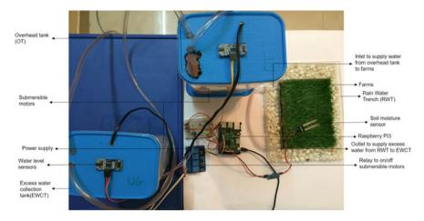
Fig. 4 Setup of smart irrigation system
