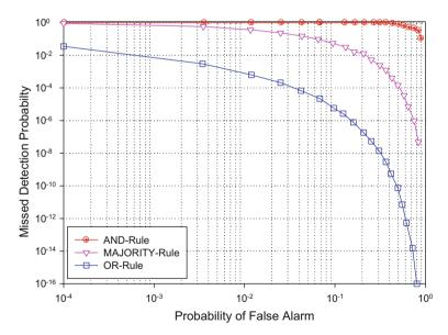
Fig. 3 CROC curves of hard fusion rule in Rayleigh channel
