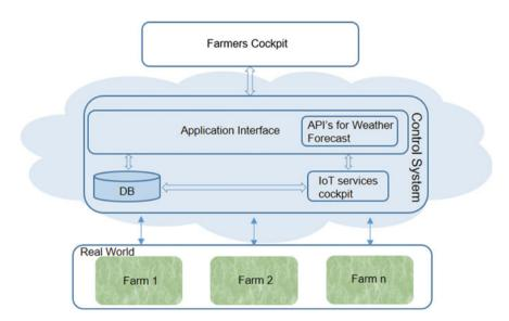
Fig. 1 Framework for smart irrigation system
