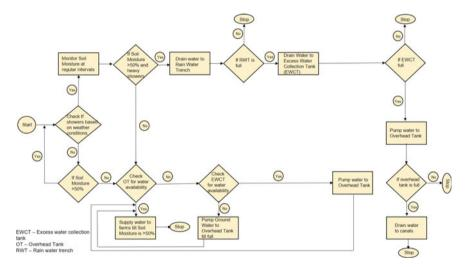
Fig. 3 Process flow for smart irrigation system
