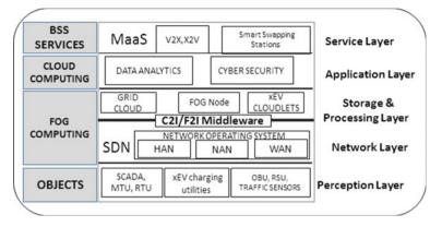
Fig. 4 Service Oriented Architecture of a Cloud-Fog system for IoT aware battery swapping/charging station
