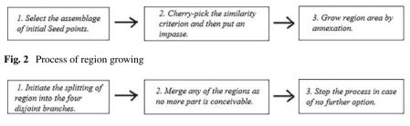
Fig. 3 Three steps of region splitting and merging
