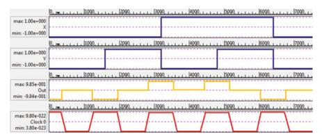
Fig. 6 Simulation waveforms for the proposed fault-tolerant XOR gate
