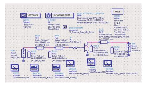
Fig. 1 LNA design with the gate resistor
