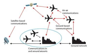
Fig. 1 Airborne ad-hoc network with both air-to-air communication and air-to-ground communications [14]
