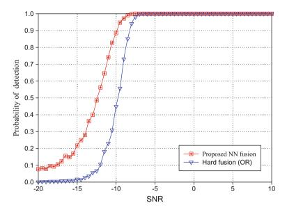
Fig. 4 Detection accuracy curves for different fusion rules for different SNR values
