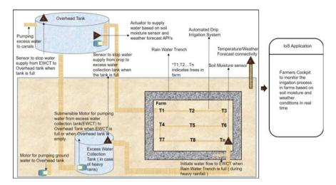
Fig. 2 Proposed smart irrigation system
