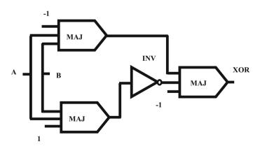
Fig. 4 Schematic of QCA-based new 2-input XOR gate
