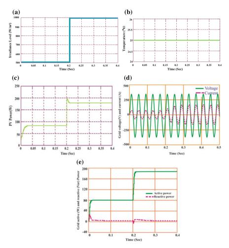
Fig. 6 Simulated responses of **a** irradiance level **b** temperature **c** PV power **d** grid voltage **e** active and reactive power
