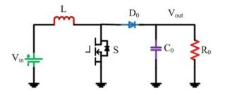
Fig. 2 Simple boost converter
