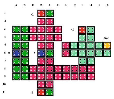
Fig. 5 QCA layout of proposed fault-tolerant 2-input XOR gate
