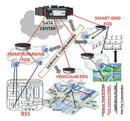
Fig. 3 Cloud-IoT architecture for intelligent Battery Swap Station (BSS)
