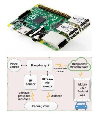
**Fig. 5** Architecture of the smart parking system
