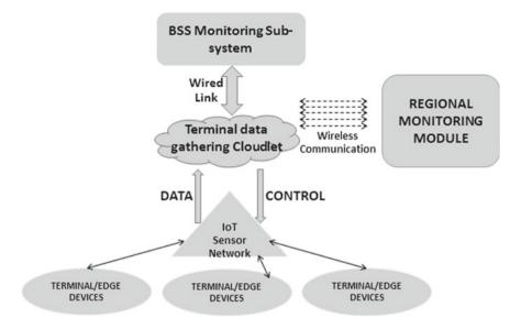
Fig. 2 Architecture of a typical IoT aware Battery Swap Station (BSS)
