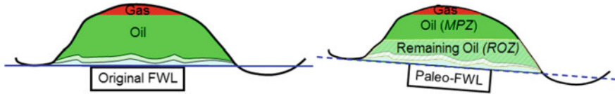
Fig. 3 Effect of tilting on initial hydrocarbon distribution
