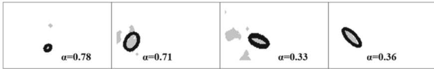
Fig. 5 Ellipses fitted on Watershed segmented pores for calculating aspect ratios; \alpha 's denote the respective aspect ratios of the pores segmented by the Watershed transform
