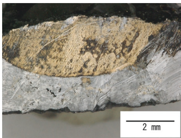
Fig. 16.4 Microscopic cross-sectional image of precipitated metal in reduction sample
